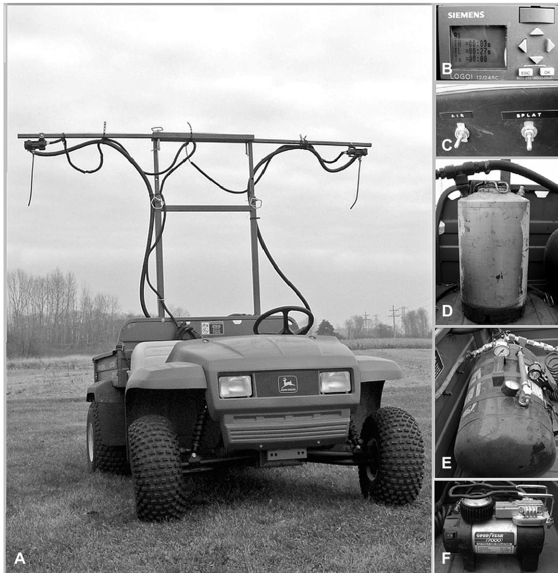
**Fig. 1.** ATV-mounted mechanical applicator for deploying drops of SPLAT-GBM in vineyards. A: steel frame, solenoids and nozzles; B: programmable timer; C: dashboard switches; D: SPLAT-GBM holding tank; E: pressurized air tank; F: electric air pump.
